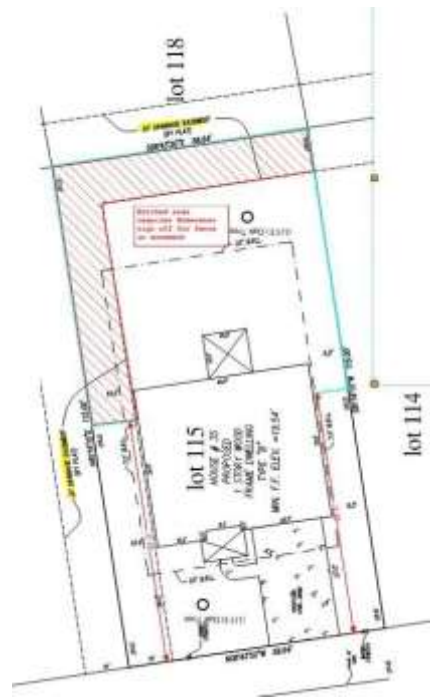
Lot with Fence in Easement
